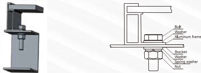
Figure 5 Bolt Installation of Mono-facial Modules
