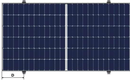
Installation of framed module with fixtures on long sides (beam perpendicular to long sides) (clamp length \geq 40\text{mm} )
