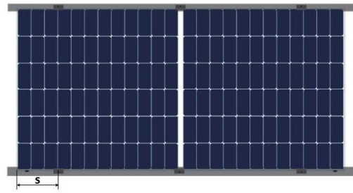
Clamps Mounting Mounting rails cross the long frame. (clamp length \geq 40\text{mm} )
