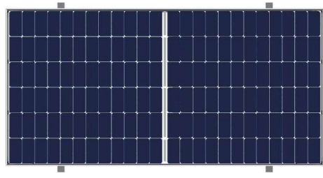
Outer Four-hole bolts Mounting Mounting rails cross the long frame.
