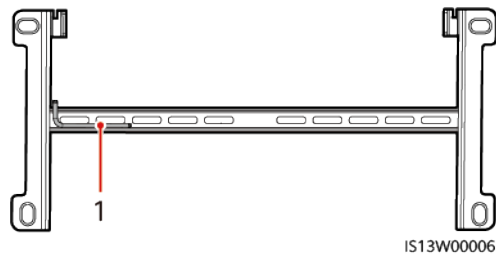
Figure 4-9 Position for binding the security Torx wrench
