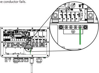
Earth Connection (Copper wires) (bypass)
