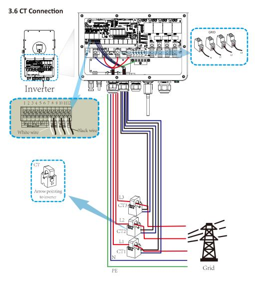
\*Note: when the reading of the load power on the LCD is not correct, please reverse the CT arrow.
