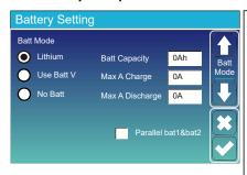
**Battery capacity:** it shows your battery bank size to Deye hybrid inverter.
